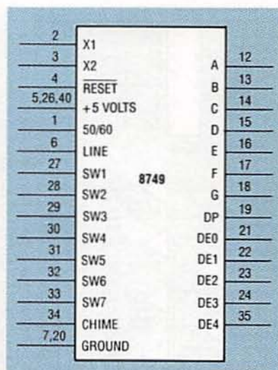
FIG. 3—THE PINS ON THE 8749 microcontroller are assigned various functions by the HyperClock program.
